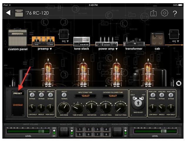
Before editing a preamp, tone stack, power amp, transformer or EQ, you might want to quickly load a preset for that module as a starting point for your edits. You can find the 'Preset' button on the left side of each module. Just tap it to load or save a module preset.
