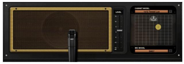
The Cab module simulates the tonal response of a guitar-amp speaker and cabinet and the microphone choice and placement on the cab. BIAS Amp's cab simulations emulate vintage, modern, bass and acoustic types of cabs.
