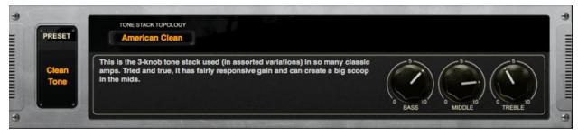
The tone stack is a specialized type of audio filter incorporated into the circuit of an amplifier for altering the frequency response of the amplifier. Tone stacks are typically placed between the preamp and power amplifier. They are the most important tonal circuit in most amplifiers.
